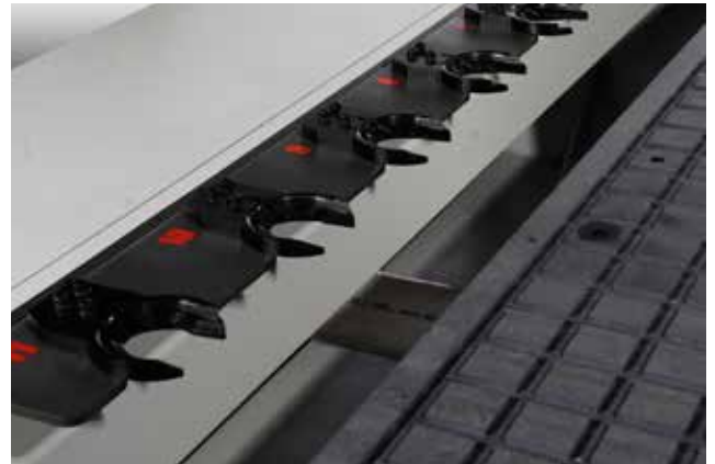
Automatic Tool Changer (ATC) Optimized for Faster Throughput
